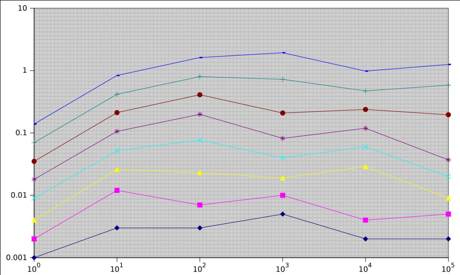
Different sizes (below) and strides (X axis) compared to their run time in sec. (Y axis) of sumArray
